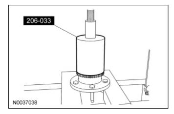
2. Install the front hub and bearing assembly. For additional information, refer to <u>Section 204-01</u>.
